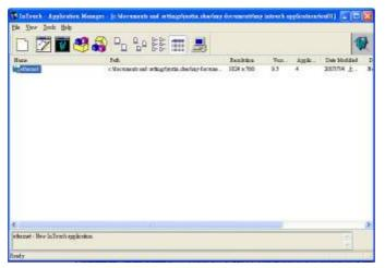
2-8. In **InTouch-WindowMaker**, go to **Configure**  $\rightarrow$  **Access Names** and double click then select on **Add** in the dialog box that appears. Enter an Access Name. The Application Name must be "**MBENET**" and the Topic Name must the same as the MBENET Topic Definition that was defined earlier (i.e. "EN01").
