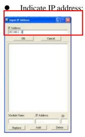
Press "IP search" button, then the input IP address window will pop out. User can type IP address in the upper space.
