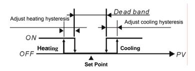
Output of defined when in PID control mode (Ctrl=PID):
